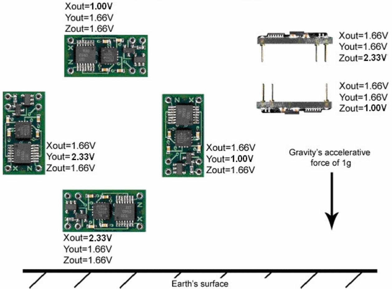
The voltage outputs on the DE-ACCM3D2 correspond to acceleration being experienced in the X, Y and Z directions. The output is ratiometric, so the output sensitivity (in mV/g) will depend on the supply voltage.
