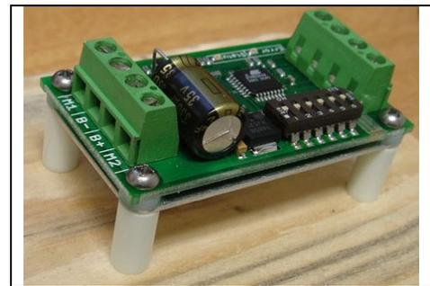
Figure 2.3: Mounted to a wood frame using standoffs
