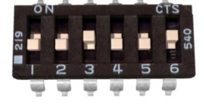
A 6-pin DIP switch assembly with pins labeled 1 through 6. The top of the assembly has 'ON' on the left and 'CTS' on the right. A blue tab labeled '219' is on the left and '540' is on the right. For Address 131, switches 1, 2, 3, and 6 are in the 'ON' position, while switches 4 and 5 are in the 'OFF' position.   |
