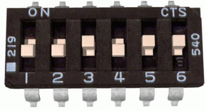
A 6-pin DIP switch assembly with pins labeled 1 through 6. The top of the assembly has 'ON' on the left and 'CTS' on the right. A blue tab labeled '219' is on the left and '540' is on the right. For Address 129, switches 1, 2, 3, and 5 are in the 'ON' position, while switches 4 and 6 are in the 'OFF' position.   |
