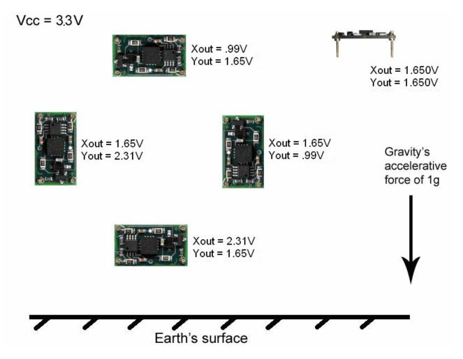
The voltage outputs on the DE-ACCM2G correspond to acceleration being experienced in the X and Y directions. The output is ratiometric, so the output sensitivity (in mV/g) depends on the supply voltage. The onboard regulator of the DE-ACCM2G2 keeps a constant 3.3V, making sensitivity a consistent 660mV/g.
