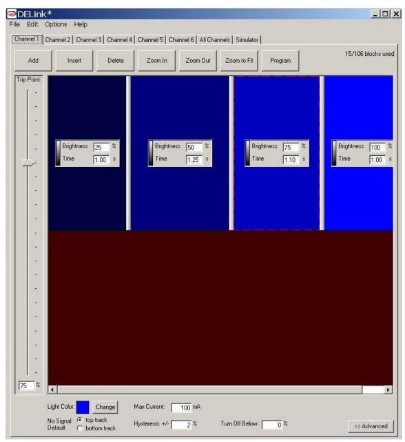
• Commands on a given channel are divided into two tracks, Top and Bottom. Which is active at any given time depends on your throttle and the Trip Point.
