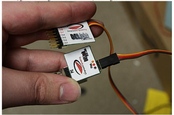
LEDs hook in as shown below, with the red wire facing the Controller label. Your computer's USB hub may not be rated for a lot of current, so only connect one LED at once when powered via USB.
