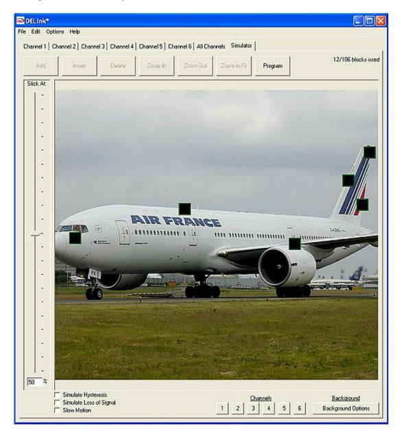
The lighting channels are represented by the black squares. Click and drag any of the channel displays to form your own patterns. Mouse over a square to see which channel it corresponds to, and right click on it to change its image from the defaul. The background can likewise be changed by right clicking it and selecting **Change Background**, which you can then fill with any image you like.
