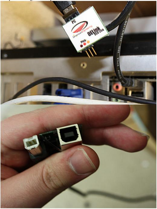
The servo connector of the DELight Controller (that would normally hook into your
