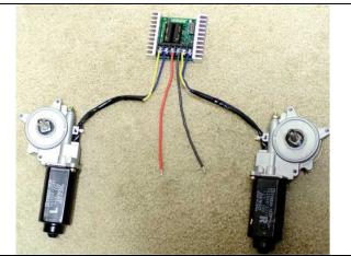
The motors connect to terminals M1A/B and M2A/B
