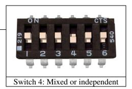
vehicle. If Switch 4 is in the DOWN position, the Sabertooth 2x25 is in Independent mode. In Independent mode, the signal fed to S1 directly controls Motor 1 (outputs M1A and M1B) and the signal fed to S2 controls Motor 2.
