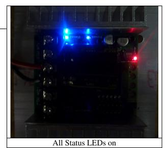
The red Error LED illuminates if the Sabertooth has detected a problem. It will light if the driver has shut down due to a depleted battery or due to overheating, overcurrent or overvoltage. If you are using a NiCd or NiMH battery, and commanding an acceleration causes the motor to jerk and the Error LED to flash on and off, the battery is depleted.
