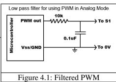
filter capacitor such as 1uf or 10uf will result in smoother motor operation, at a cost of slower transient response. A PWM frequency higher than 1000Hz is recommended.
