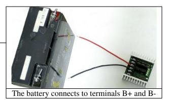
connect the battery through a connector instead of directly to the motor driver. This makes it easy to unplug the battery for charging, and prevents plugging in the battery backwards.
