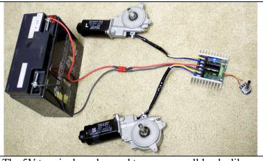
The 5V terminal can be used to power small loads, like a potentiometer or a radio receiver. The 0V signal must be connected to the ground of the device generating the input signal.
