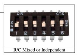
When switch 4 is in the DOWN position, Independent mode is selected. In this mode, the signal fed to the S1 input directly controls Motor 1 (M1A and M1B) and the signal fed to S2 controls Motor 2.
