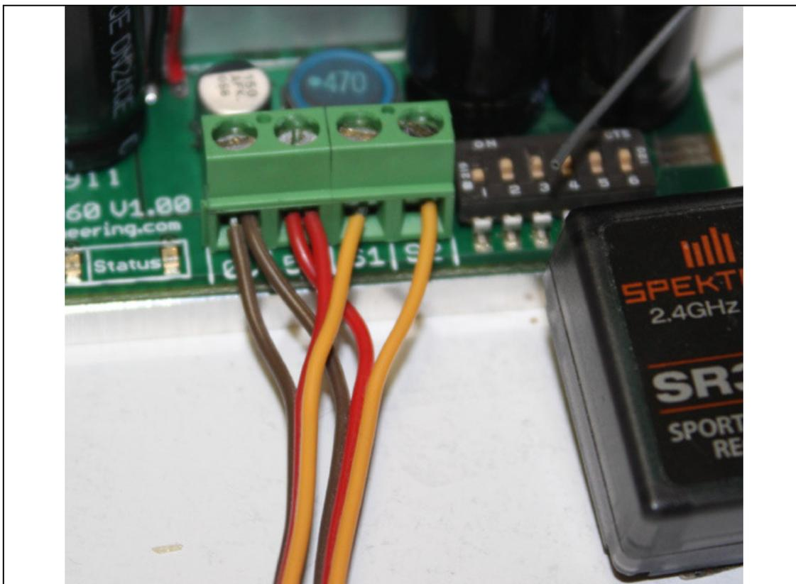
Figure 5.1: R/C connection. Each pigtail is connected to 0V, 5V, and either S1 or S2. An example connection would be the S1 pigtail to elevator and the S2 pigtail to aileron.
