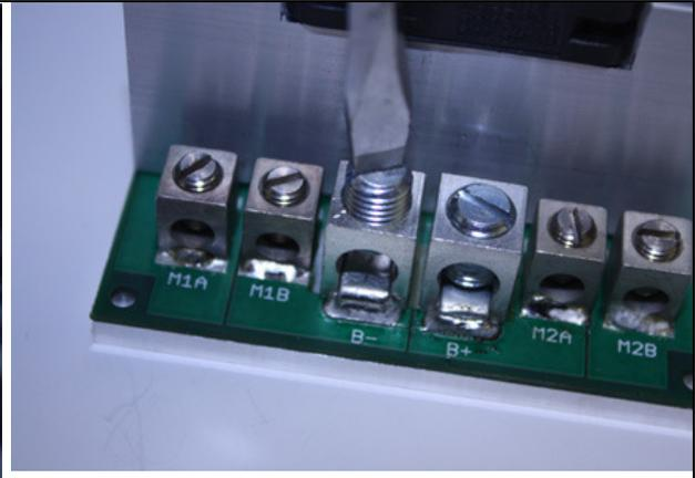
**Step 2:** With a medium sized screwdriver, turn the top screw counter-clockwise until there is enough clearance to fit the wire.
