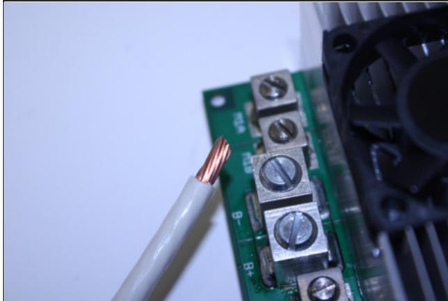
**Step 1:** Strip the wire which you are using approximately  $\frac{1}{4}$ ". Use thicker wire for high current applications. *See the chart on the next page for wiring guidelines.*
