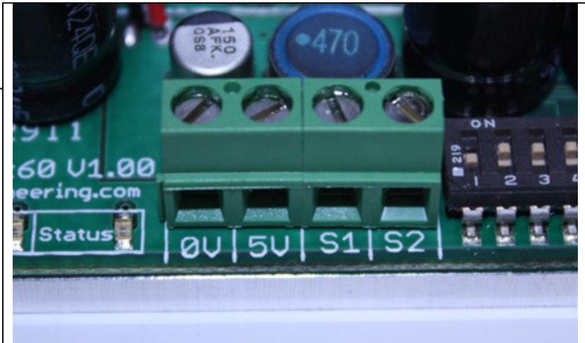
The 5V terminal can be used to power loads up to 1A continuously and 1.5A for peaks. The 0V signal must be connected to the ground of the device generating the input signal.
