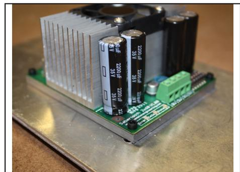
Figure 2.3: Mounted directly to a metal frame
