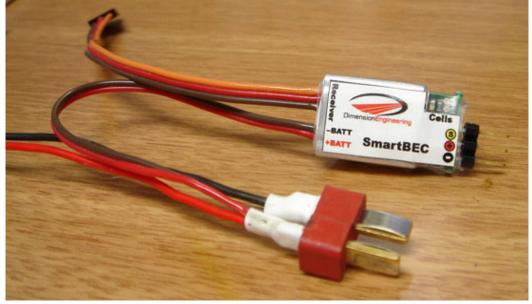
**Step 3:** Plug the radio connector of the **SmartBEC** into the throttle port of your receiver.
