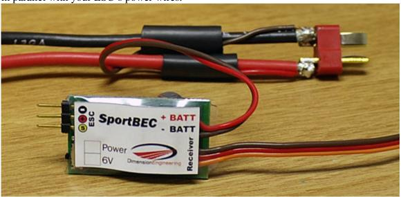
It is good practice to seal the battery connections with heatshrink tubing.
