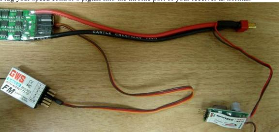
**Step 3:** Plug SportBEC's pigtail into the battery port of your receiver, or any other empty channel.
