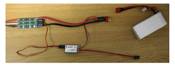
**Step 3:** Plug the radio connector of the SportBEC into the throttle port of your receiver (usually channel 3).
