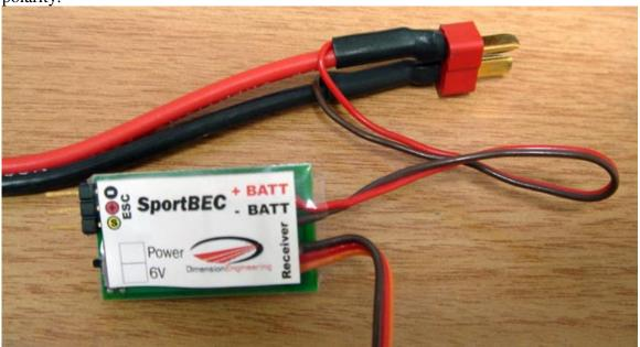
**Step 2:** Plug your speed control's pigtail into the throttle port of your receiver as normal.
